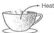
Heat always flows from hotter objects (hot drink) to cooler ones (air).
